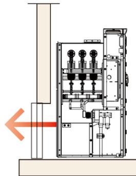
The total hole size is not less than 0.5m
