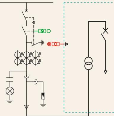
Circuit breaker cabinet locks the low-voltage side circuit breaker of transformer (two locks and one key)
