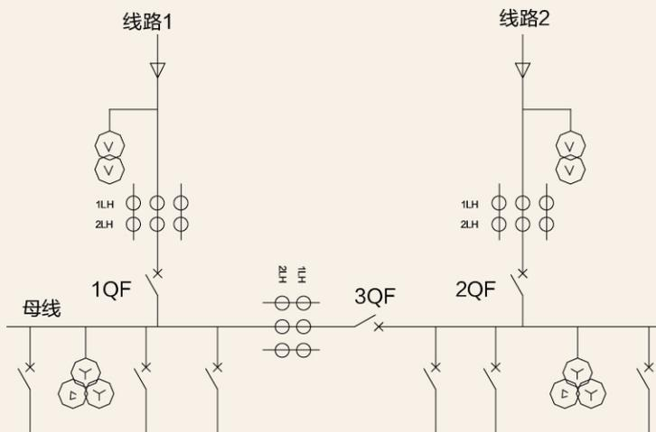
Power switching between 2 incoming lines (1QF and 2QF) and bus tie switch (3QF). 4 working modes (can be selected from the MIC500 unit)
