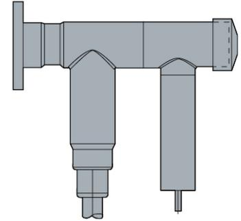
Front plug and arrester assembly drawing
