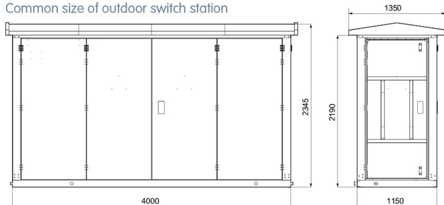
Outdoor box width: The sum of the width of a single ring network cabinet + DTU width (standard 600mm) + reserved space (400mm)
