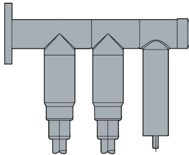
Assembly drawing of front plug, rear plug and arrester
