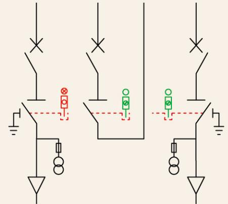
Locking transformer door of circuit breaker cabinet (two locks and one key)
