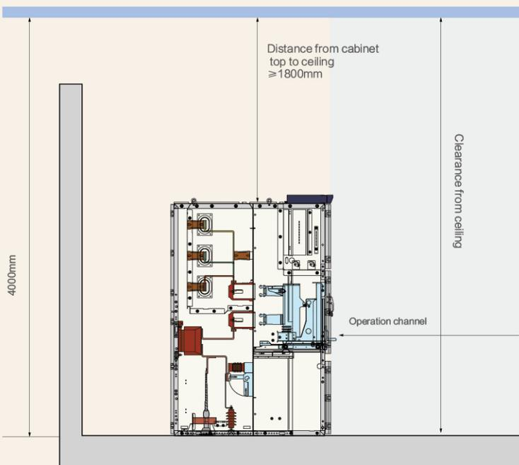
Minimum operating clearance channel in front of the switch cabinet when the switch cabinet is against the wall (m)
