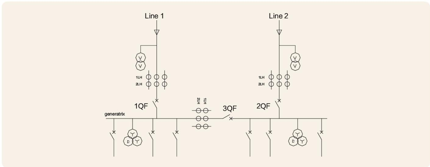
Power switching between 2 incoming lines (1QF and 2QF) and bus tie switch (3QF). 4 working modes (can be selected from the MIC500 unit)
